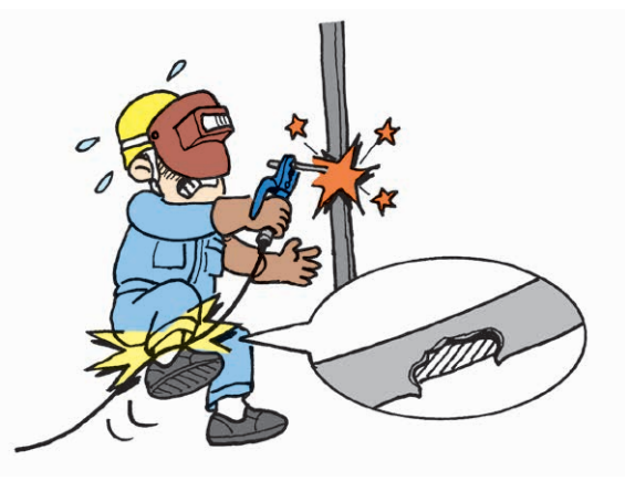
Electric shock due to exposure of secondary side wiring of an arc welding machine
